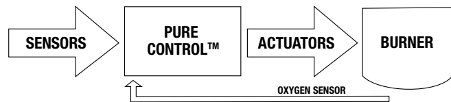
▲ Fig 3. Closed Loop O 2 Compensation
